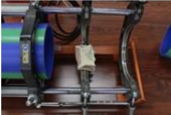
Shimming Front Clamp
