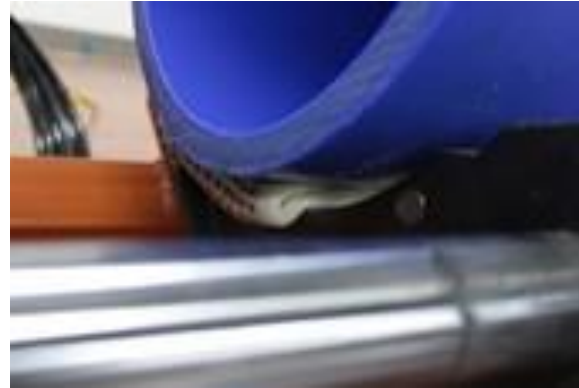
Shimming Front Clamp
