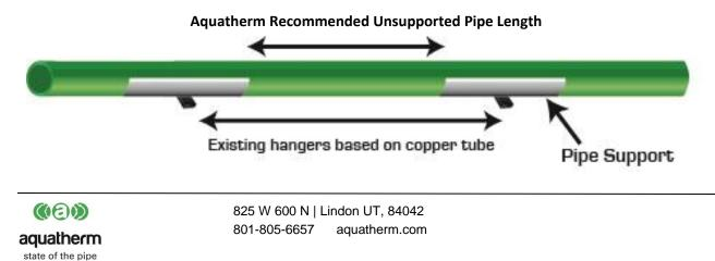
The example table below gives the length of each size of pipe reinforcement for each pipe diameter along with the resulting minimum hanger spacing. Also in the table is the typical hanger spacing allowed for copper tube.
