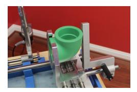
In some cases, there are modified clamps that reduce the compressive effect on the fitting. If the issue persists, contact the manufacturer of the tool to see what options are available.
