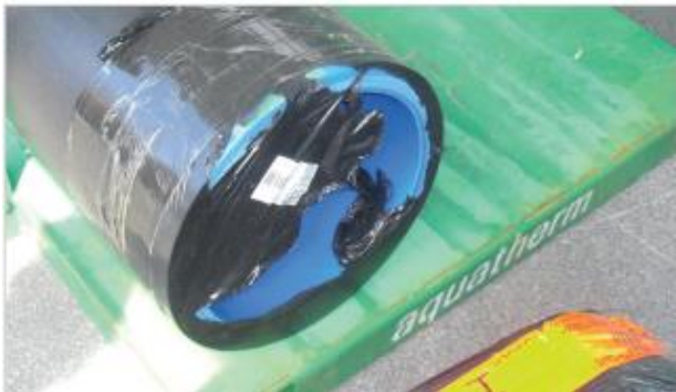
Figure 3 Possible damages caused by container loading.
