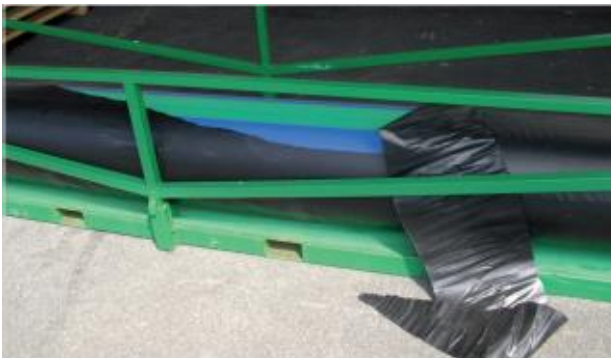
Figure 5 Possible tearing from container loading.
