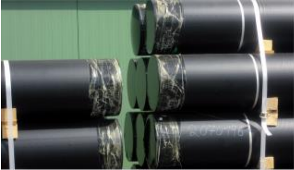
Figure 1: Sealed pipe ends.
