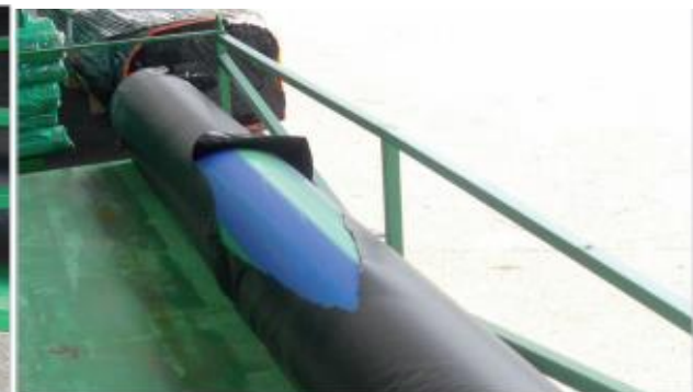
Figure 6 Possible tearing from container loading.
