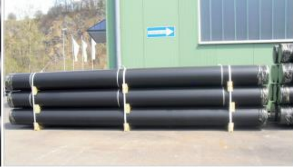
Figure 2 Outdoor Storage with film in good condition.
