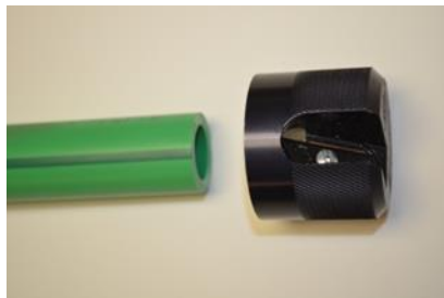
Chamfer tool and pipe
