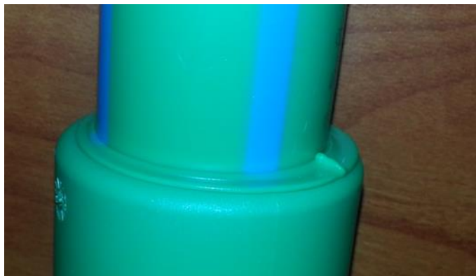
Flat fusion bead from use of cold ring.
