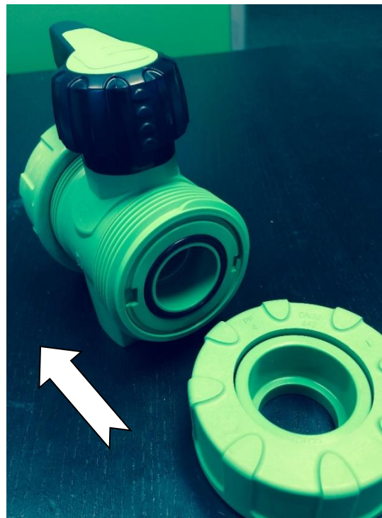
Figure 1: Aquatherm Polypropylene Ball valve showing access to the valve ball and internal parts. It is suggested to install the valve with flow in the direction of the arrow.
