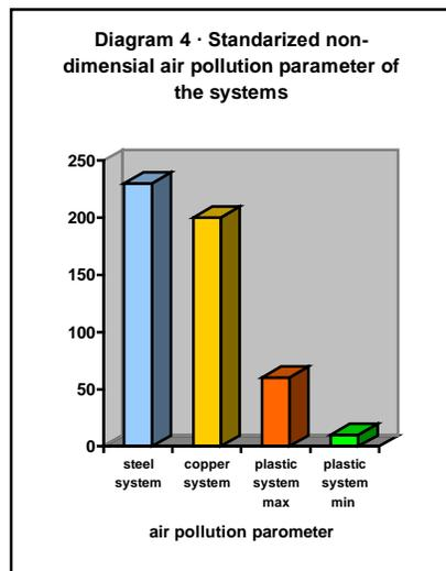
In diagram 4 the metallic systems of galvanised steel and copper represent one group with the two plastic system categories of "Min" and "Max" forming the limits of the second group. The steel and copper pipe systems show high absolute values in a large number of emissions.
