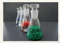
Polypropylene is a fusible thermoplastic. It is clean enough to use in distilled water systems and strong enough for use with acid waste. Our polypropylene resin has been developed specifically for pressure piping applications and will outlast and outperform other piping materials.
