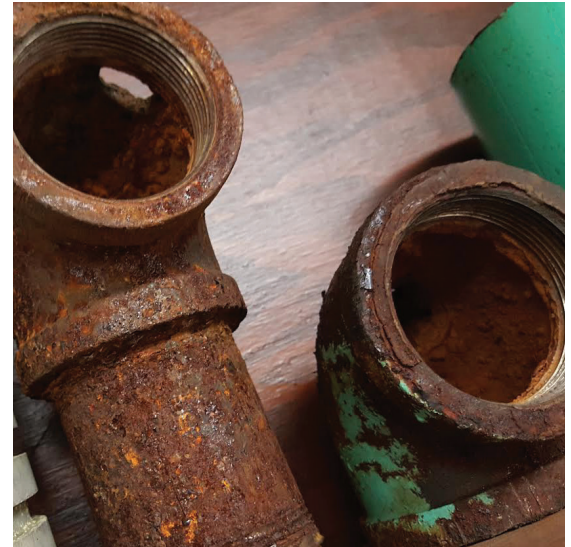
Polypropylene pipe is hydrophobic and will never scale and corrode the way metal pipe does.
