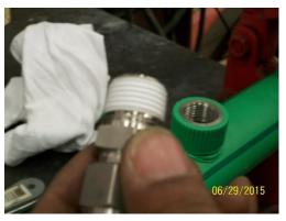
Apply 2 wraps of ½" PTFE tape (e.g. Teflon®). Holding the fitting in your left hand with the Male threads facing away from your hand, apply the 2 wraps of PTFE tape in a clockwise rotation as shown in the photos above.
