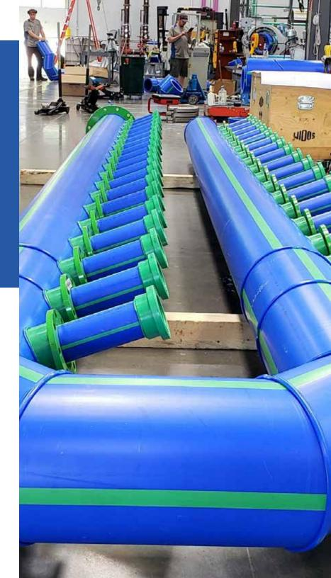
In addition, the ability to prefabricate polypropylene pipe offers a huge advantage in time- and labor-savings over metal pipe. For example, risers can be custom fabricated for the existing space with all the tees already in place. As MacNevin notes, "For every tee you can prefabricate on the workbench, that's three joints that you don't have do in a confined space."
