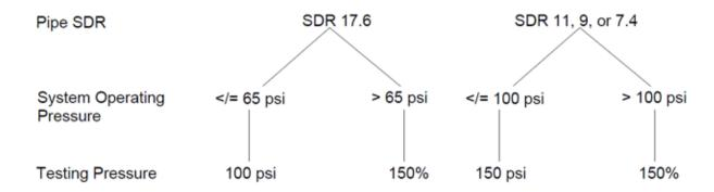
The following are maximum testing pressures for high-rise buildings or high-pressure systems. The maximum testing pressures should not exceed the following:
