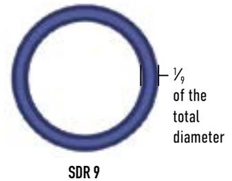
A heavy wall provides increased temperature and pressure capabilities for higher stress applications such as mechanical hot water systems.
