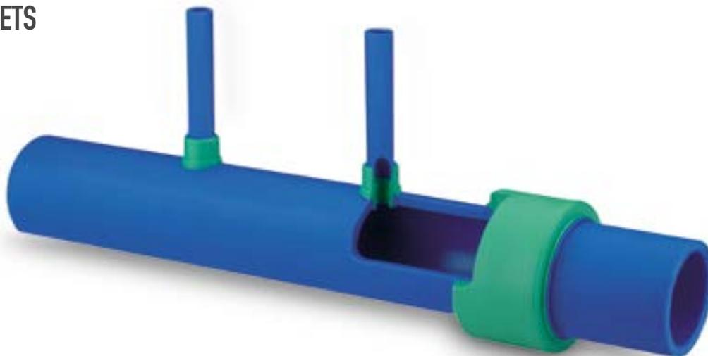
For installations with branch lines, fusion outlets offer many advantages over traditional reducing tees. Fusion outlets are installed directly onto the side of the pipe and can be added after the main lines are already in place. Fusion outlets also generate less friction than a reducing tee, lowering the pressure loss of the entire system.
