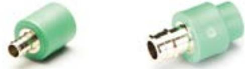
Featuring a PP-R/PP-RCT fitting on one end and a barbed brass end for PEX tubing, these transitions offer a simple solution for installing a system with both PP-R/PP-RCT and PEX for 1/2", 3/4" and 1" sizes.
