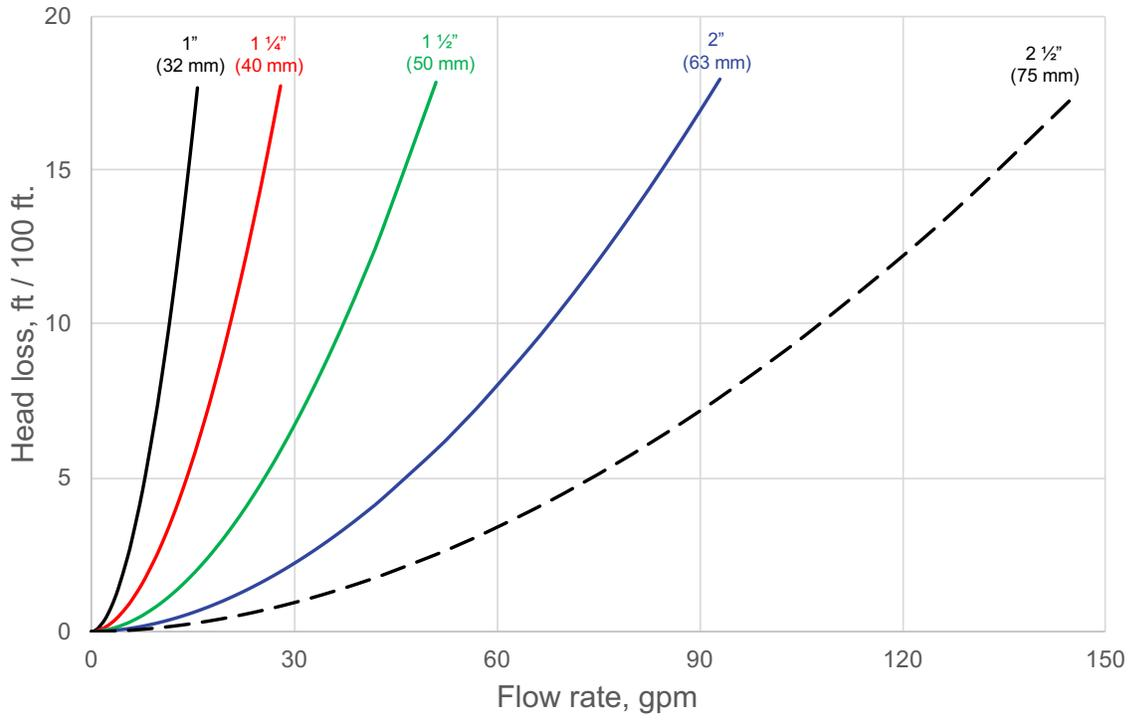
Pressure Loss vs. Flow Rate
