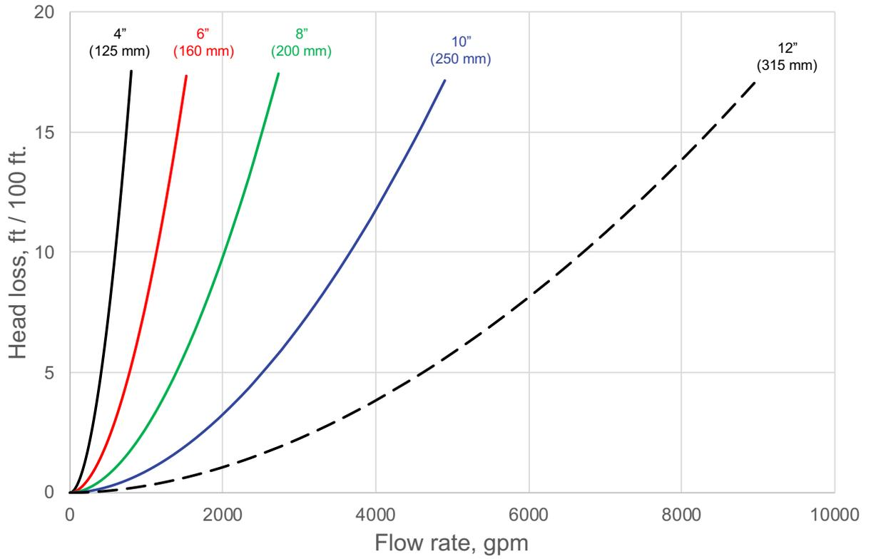
Pressure Loss vs. Flow Rate
