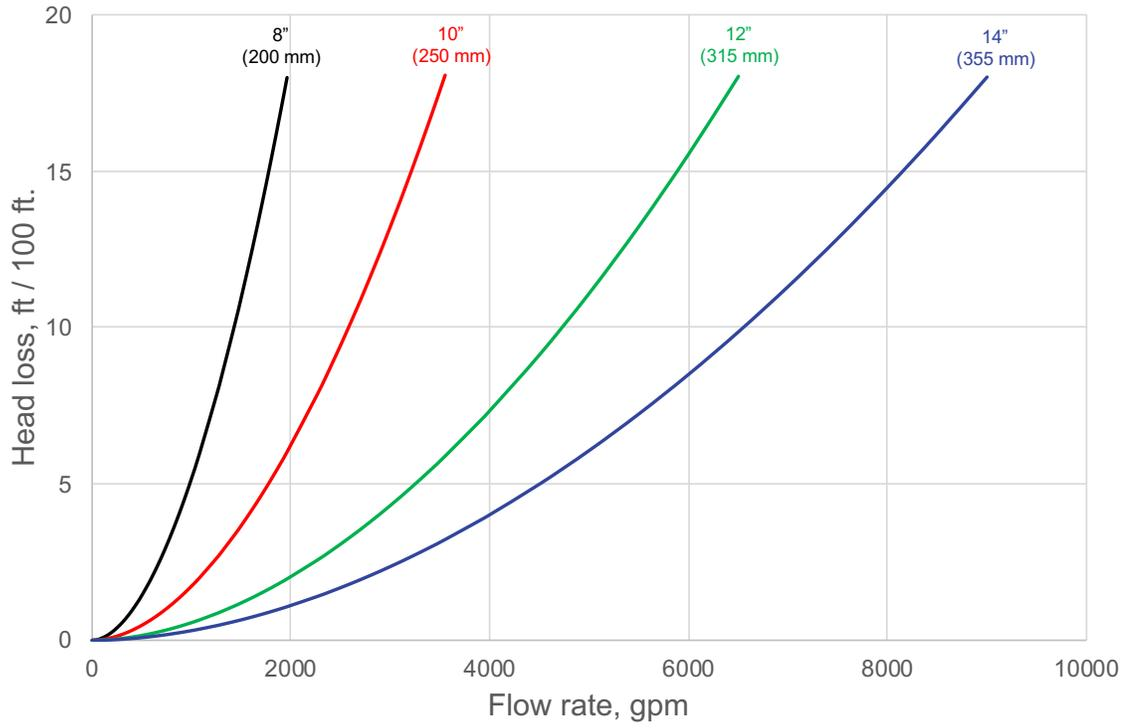
Pressure Loss vs. Flow Rate
