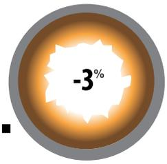
Corrosion and scaling can reduce the inside of steel pipes by an average of 3% per year, resulting in lost efficiency and up to 10% increased pumping energy annually. This can add up to thousands of dollars in hidden energy costs over the life of the system.
