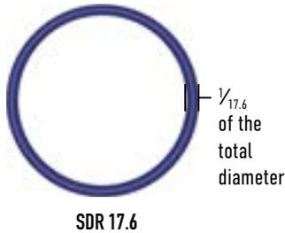
A thinner wall provides maximum flow rate while minimizing material weight, cost and fusion times. For chilled, cooling and condenser water applications.
