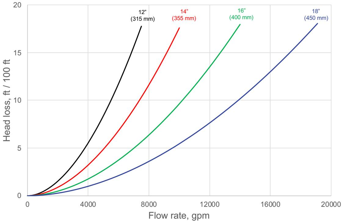
Pressure Loss vs. Flow Rate
