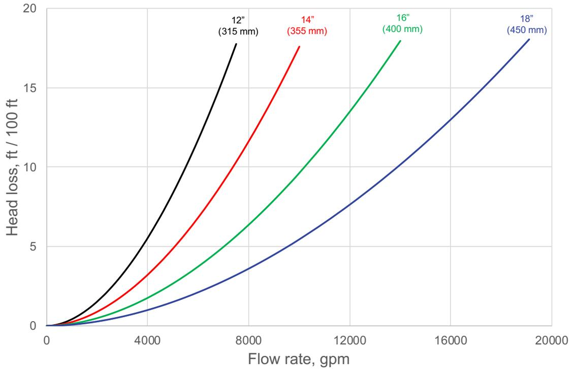
Pressure Loss vs. Flow Rate
