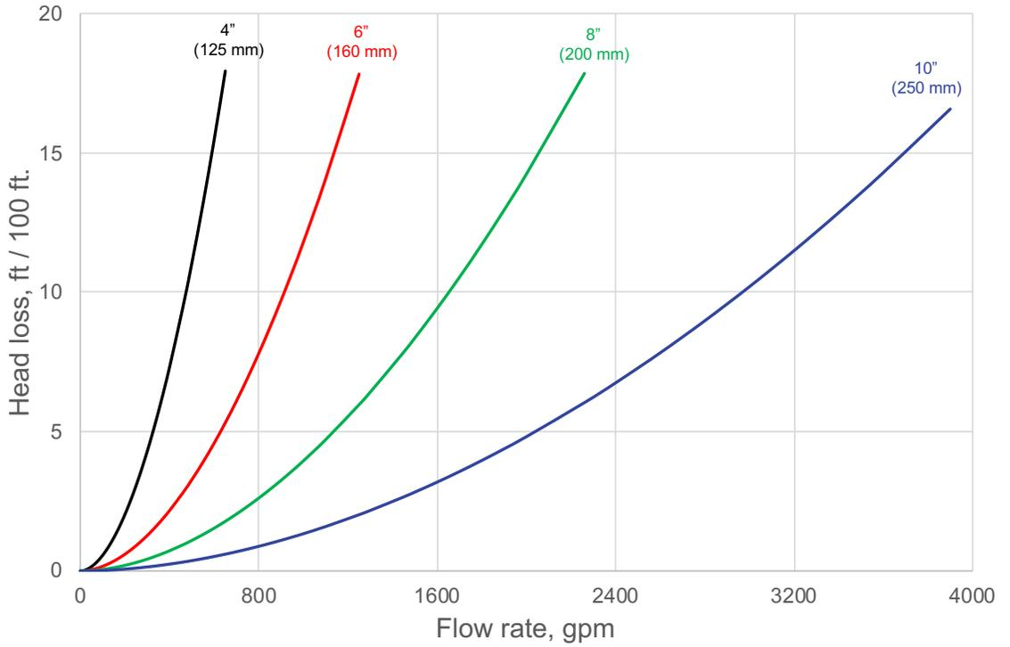
Pressure Loss vs. Flow Rate
