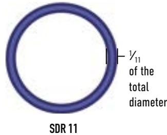
A medium wall thickness to provide higher flow rates while maintaining high pressures. Suitable for most applications.
