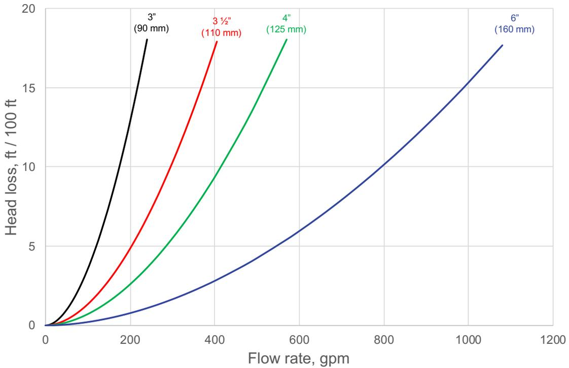
Pressure Loss vs Flow Rate
