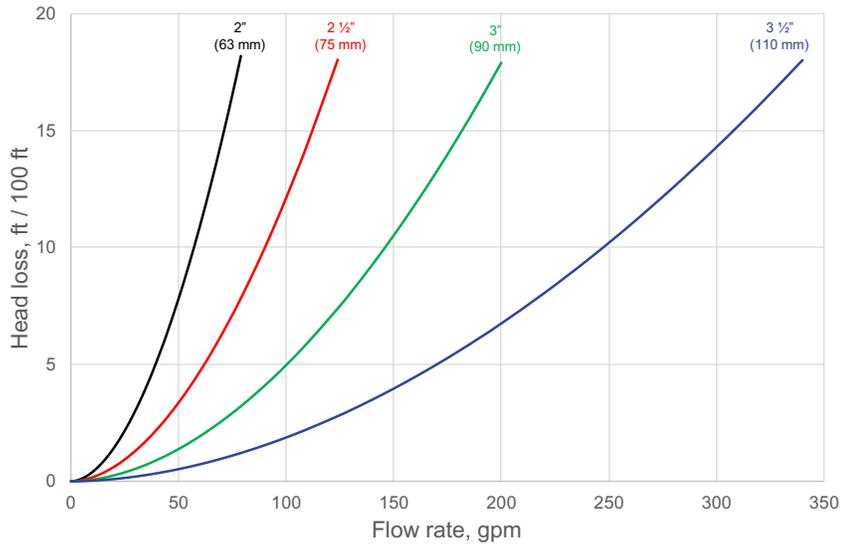
Pressure Loss vs. Flow Rate
