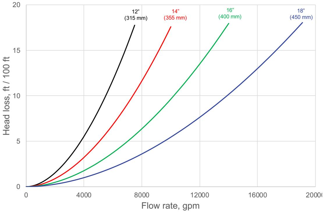
Pressure Loss vs. Flow Rate
