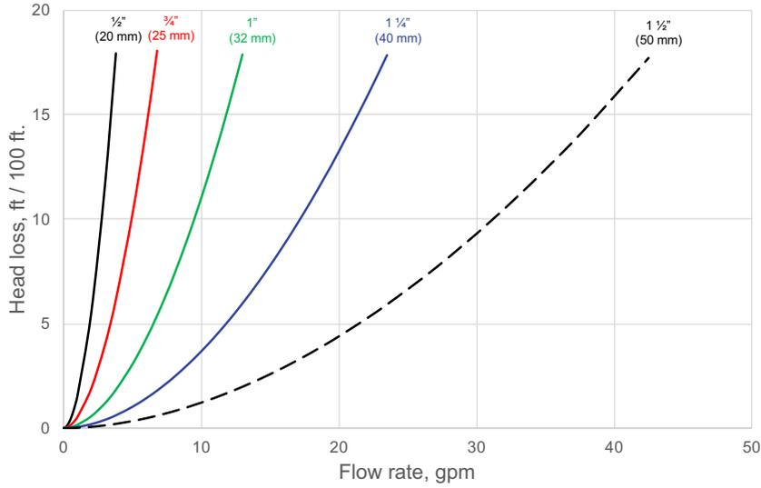
Pressure Loss vs. Flow Rate
