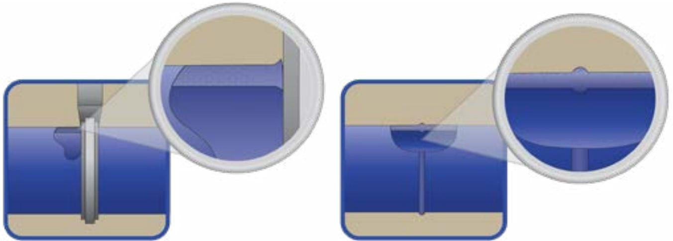
All Aquatherm piping products are made from the same reliable polypropylene material and are engineered to be heat fused together.
